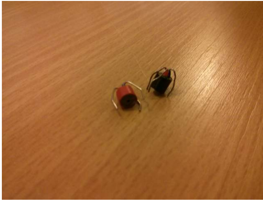
Figure 4.2: Microphone capsules used for recording, same model as the ones used for testing the phantom power supply
