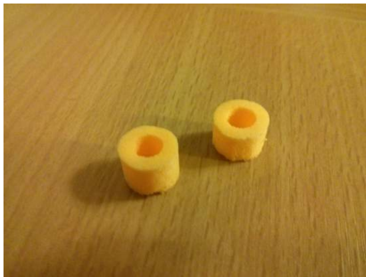
Figure 3.13: Sponge covers for the microphone capsules
