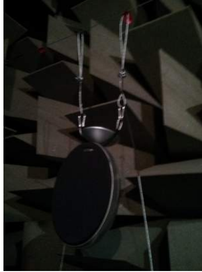
Figure 3.5: Details of one of the loudspeakers hanging from the wire
