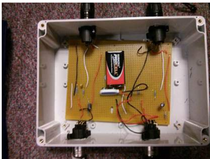
Figure 3.25: Finished version of the phantom power supply circuit
