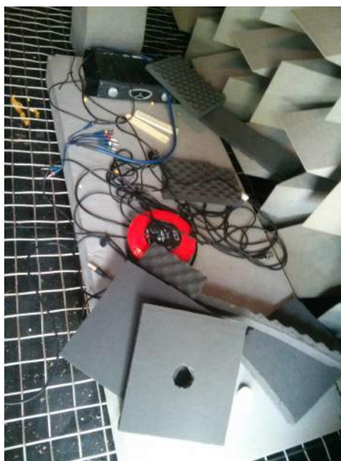
Figure 4.15: Reflective material in the anechoic chamber
