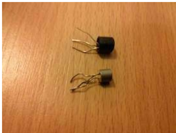
Figure 3.20: 3-Pin Electret microphone capsules used for testing
