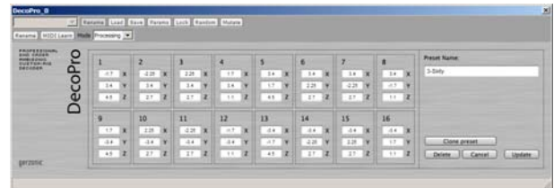
Fig. 14 – Decopro feeding 16 loudspeakers for the 3-Sixty room
