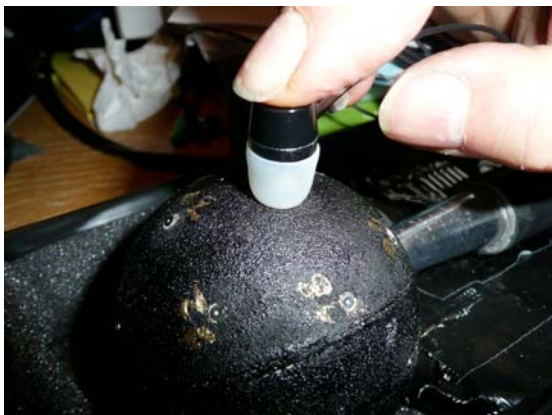
Fig. 4 – calibration of the DIY spherical microphone by means of an earplug
